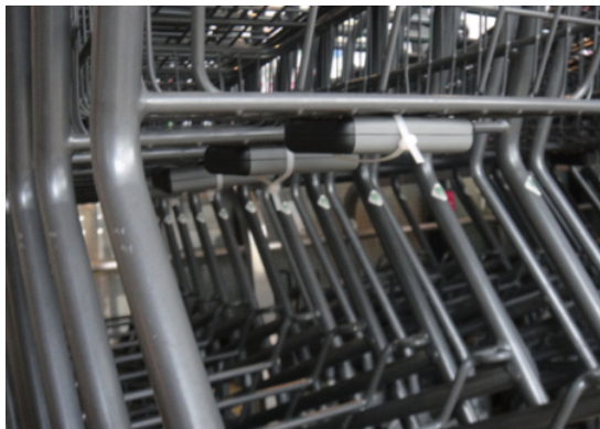
Fig. 5: RFID Antenna on a Shopping Cart
