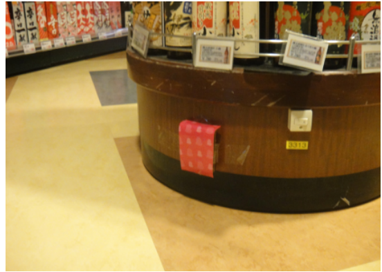
Fig. 6: RFID Antenna on a Display Fixture
