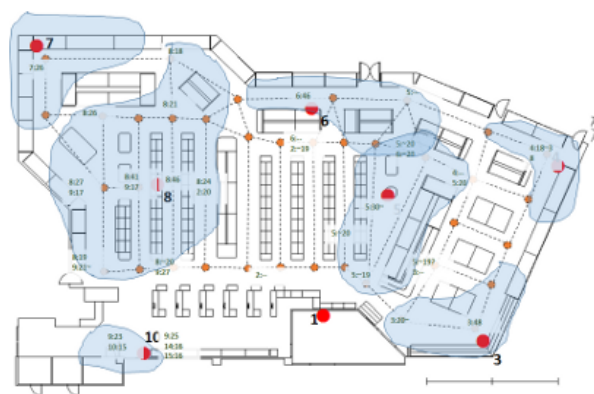
Fig. 8: Communication range of antenna
